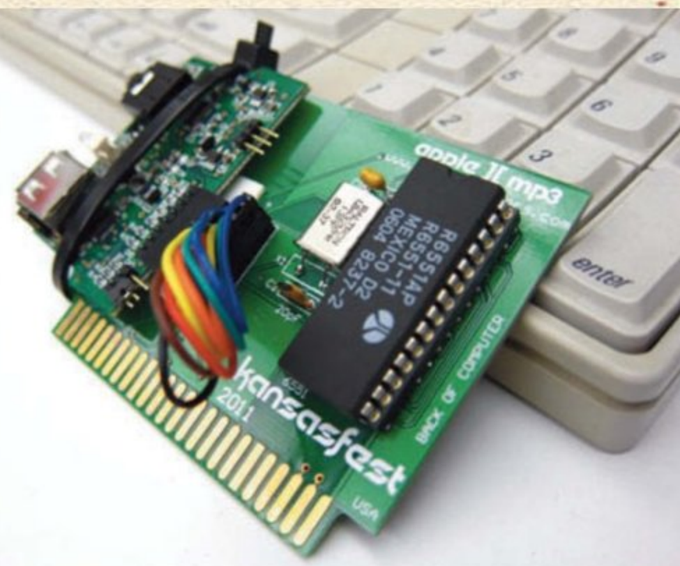
» Clever people continue to push the Apple II way beyond its original boundaries; here's Vince Briel's Apple II MP3 card, for playing back MP3s from a flash pen drive. (Photo: Andy Molloy)
